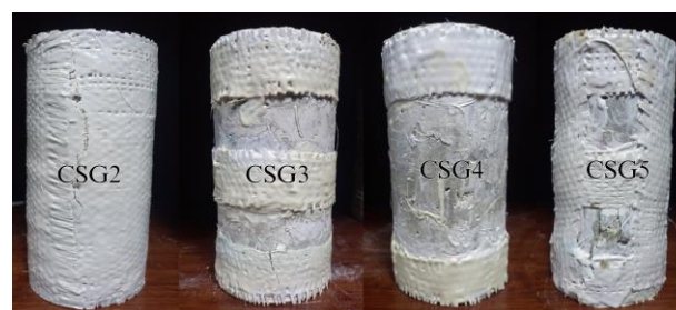
Figure 5. Failure modes of HSGFRP wrapped circular concrete
